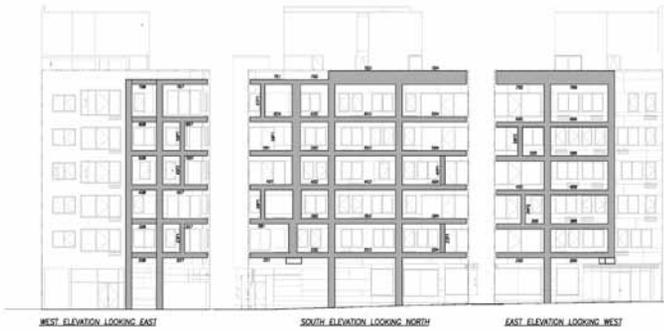
Figure 3. Unfolded elevation of the Vierendeel truss.
